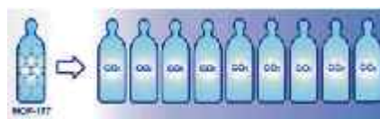
(A tank filled with the material known as MOF-177 can hold as much carbon dioxide as nine tanks that do not contain MOF-177)
